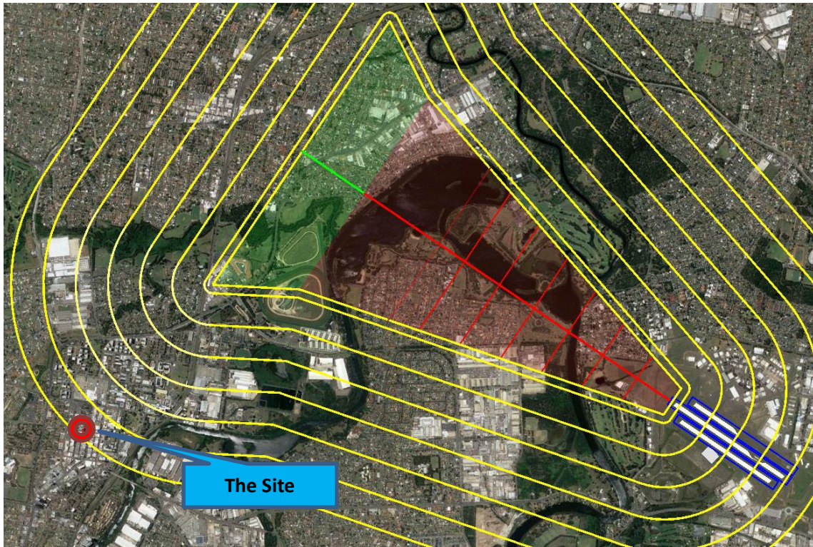
Figure 3: PANS-OPS based on calculations incorporating the Nov 2020 ICAO PANS-OPS update
